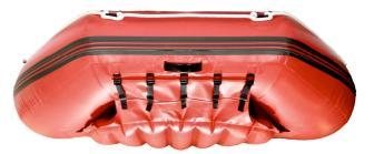
Floor at stern is adjustable for highest speed
